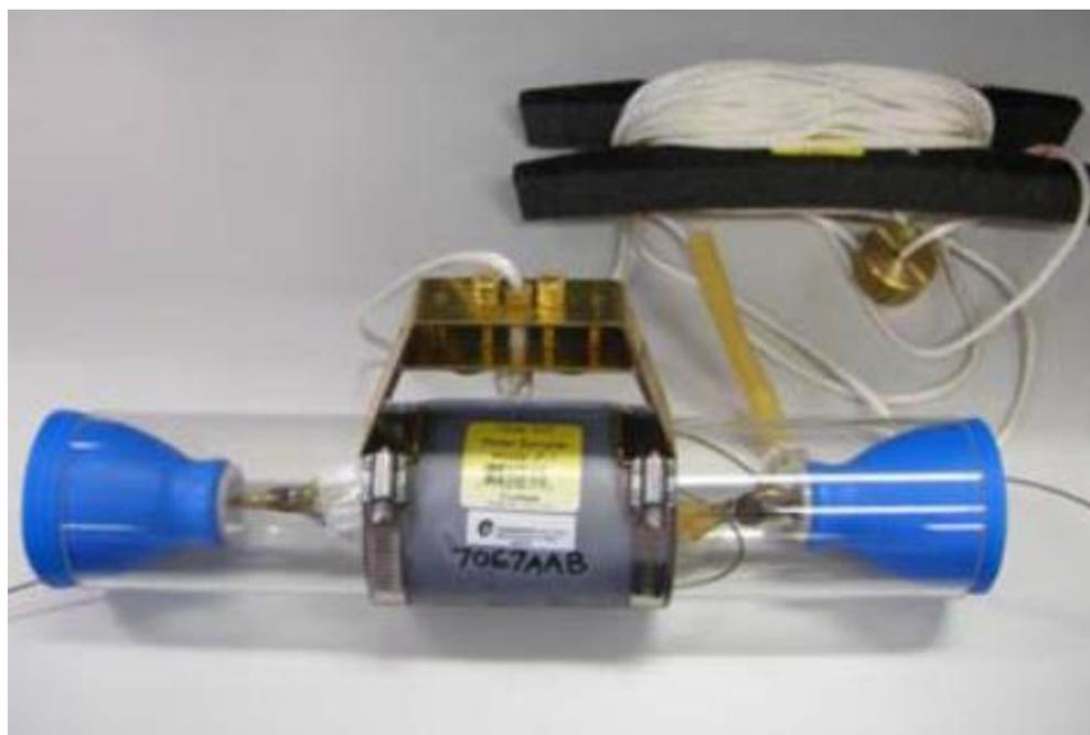
Figure 2: Van Dorn sampler
