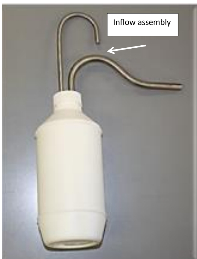
Figure 3: Stage sampler bottle with inflow assembly
