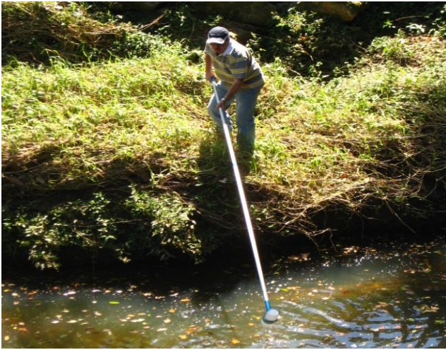
Figure 2: Using an extendable pole type sampler
