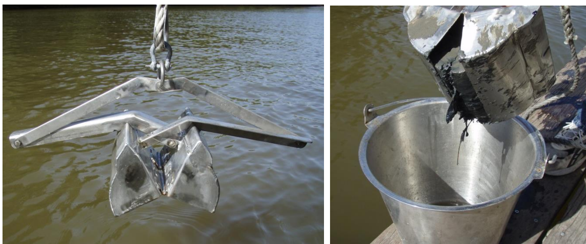
Figure 5: Van Veen Grab Sampler collecting benthic mud in sample container
