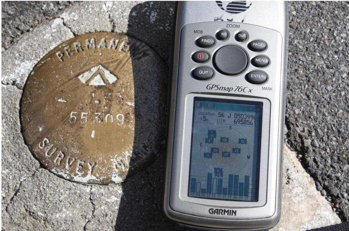
Figure 1: GPS next to permanent survey mark 55309
