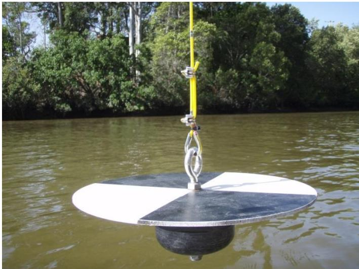
**Figure 1: Secchi disc attached to 3kg weight and tether**
