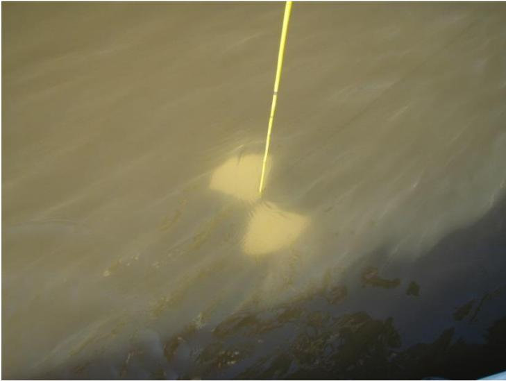
**Figure 2: Secchi disc being lowered into the water**
