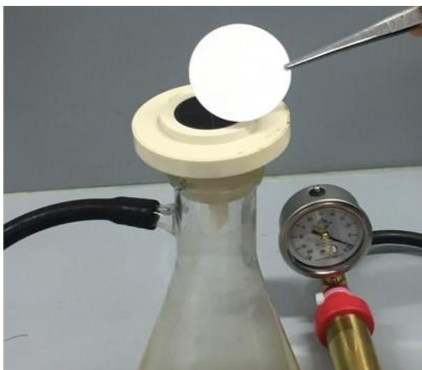
**Figure 2: Filter paper being placed into filter holder**
