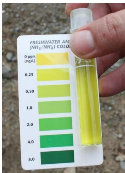
Figure 1: Freshwater ammonia test kit including tested water sample in vial and colour chart
