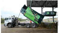
Waste is received, tipped, stored and shredded in an undercover area that has open sides. The content of food in the 'FOGO' feedstock is supplemented (or increased) by commercial sourced food waste that is blended with kerbside FOGO prior to mixing.
