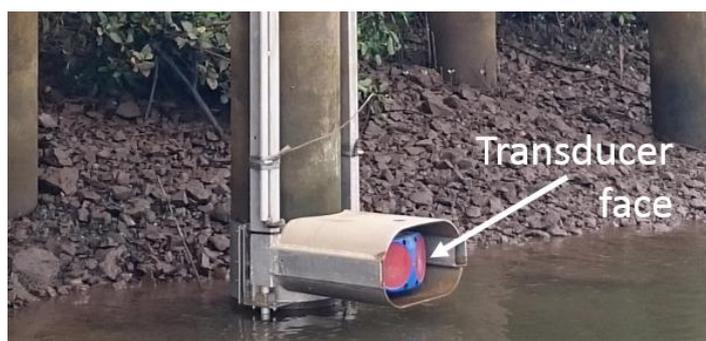
Figure 1: Example of a horizontal Acoustic Doppler Current Profiler
