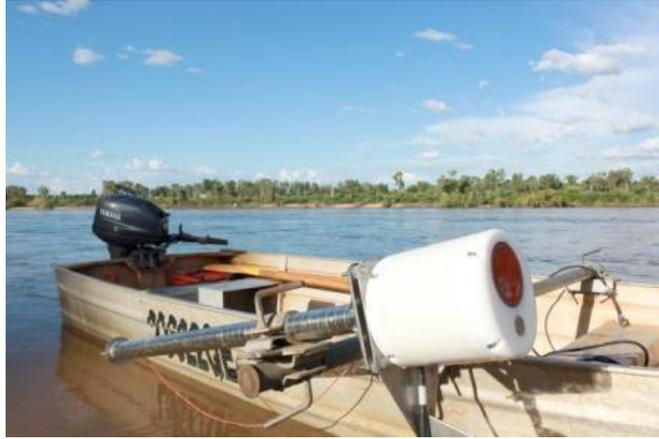
Figure 4: A boat-mounted ADCP prepared to collect velocity data
