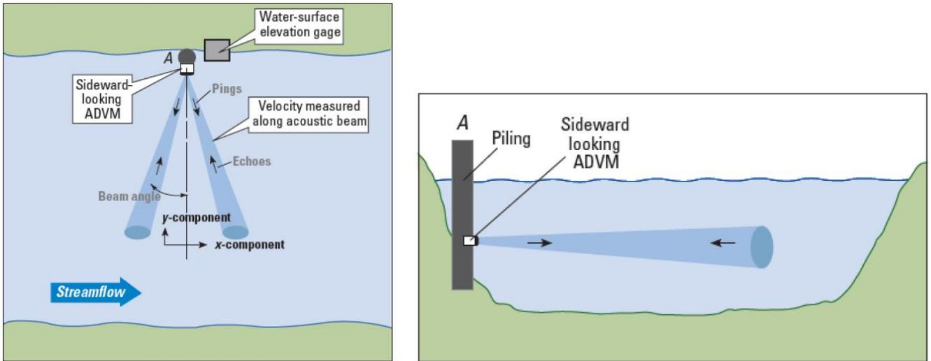
**Figure 2: Bird's eye view (left) and channel view (right) - illustration of a horizontally mounted ADCP installation (Source: Ruhl and Simpson 2005)**
