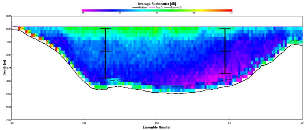
**Figure 5: A channel profile showing the spatial variation in the measured backscatter intensity using a boat mounted ADCP. The black bars represent the three locations in each vertical where grab samples must be collected to accurately calibrate backscatter intensity with TSS concentrations (Source: Mark Randall, Department of Natural Resources and Mines, QLD)**
