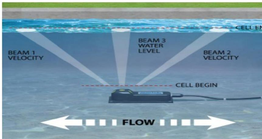
**Figure 3: Illustration of a typical bed-mounted ADCP installation (Source: Sontek/YSI Argonaut product brochure, 2009. [www.sontek.com/pdf/brochures/Argonaut-SW-2009-06-23.pdf](http://www.sontek.com/pdf/brochures/Argonaut-SW-2009-06-23.pdf))**
